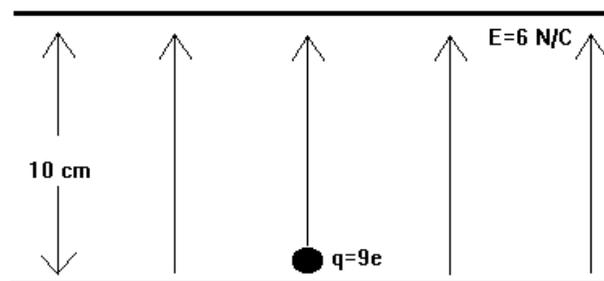
What we see from this is very simple. In a uniform electric field, the work done is simply force times (parallel) distance.
