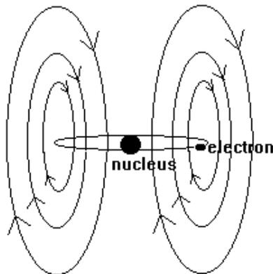
The field in this instance looks like concentric, misshapen "donuts". This shape is very, very important. The field produced in this way is called a dipole field. Notice the resemblance to an electric field created by a positive and negative charge separated by a short distance. That particular field looked this:
