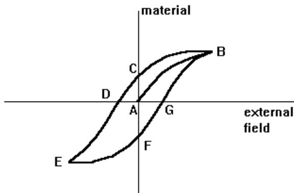
In this diagram, we begin a point A where there is no external field, and no magnetism in the material. The segments from there represent:
