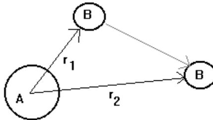
If A and B are charged particles, and B is moved from  $r_1$  to  $r_2$  along the gray line, some work (either positive or negative) is done and thus there is some energy change. However,  $qEd$  is not applicable, since the field is not uniform. In order to solve this problem, a new concept is introduced in exactly the same manner as it was when we hit the same brick wall discussing gravity. The electric potential energy of a particle at a point is given by the following equation:
