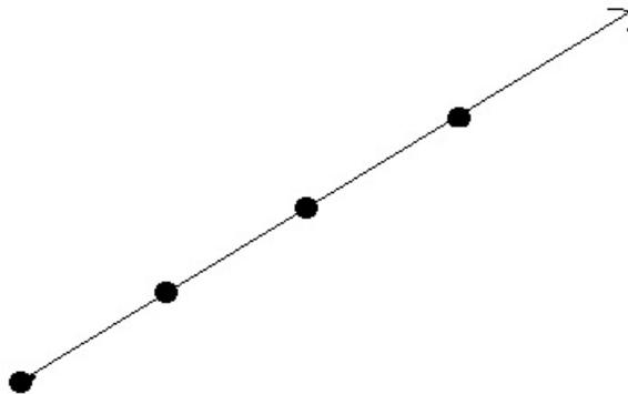
Since we know that the particle will deviate from this the same amount as the dropped object (or the horizontally thrown object), we can immediately draw the path of the projectile.
