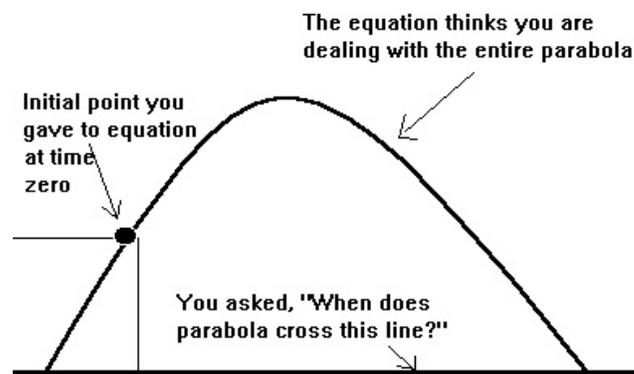
Another way to think about this mechanistic aspect of mathematical equations is that the two equations being used describe a general parabola, without beginning or end. Inputting initial conditions (initial velocity and acceleration) "pick" out a specific parabola from the infinite number of possibilities. The solution tells you the coordinates of a specific point on the parabola (for example, in the case above the equations told you that the parabola has two points where  $y=-100$  m).
