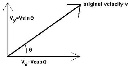
Once that is accomplished, we treat the x and y directions independently, using  $V_x$  as the initial velocity in the x direction (which will remain unchanged) and  $V_y$  as the initial velocity in the y direction (which will change according to the acceleration due to gravity). In this case, we have two motions, one of an object thrown upwards and the other of an object moving to the side at constant velocity. Combining these two motions gives a diagram like the one below.
