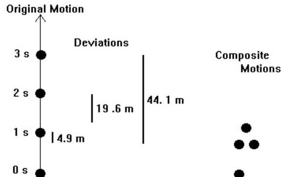
In this diagram we can see how the deviations become so much greater than the positive gains made by the constant velocity, that the particle begins to descend.
