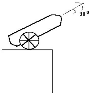
In order to solve this problem, the student should be aware of the necessity of superimposing a coordinate system onto the motion. It is typical for the origin to be at the top of the cliff (or more accurately, at the point where the free-fall begins as the ball leaves the cannon). This helps us keep our signs straight and it gives readily recognizable meaning to our negative answers.
