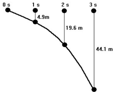
The previous example was just a restatement of what was said before. However, consider the case of a projectile fired at some angle. The intended straight line (constant velocity) path would then resemble the diagram below.
