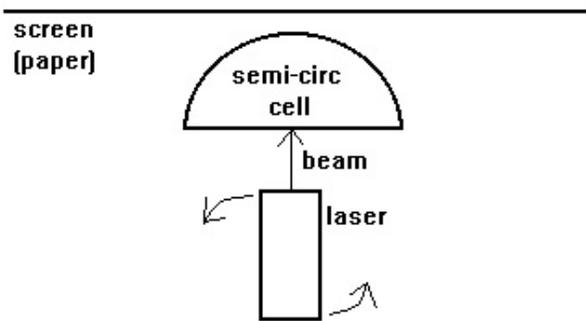
Repeat with circular part of cell towards laser. This time rotate cell around its center.
