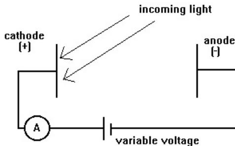
Imagine for an instant that the variable voltage was set at zero. In this case, electrons would come off the cathode (made of metal) and reach the anode. This would create an electrical current that would be measured by the ammeter. In this case, the
