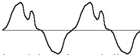
**An example of a composite wave produced by two pure tones sounded together**
