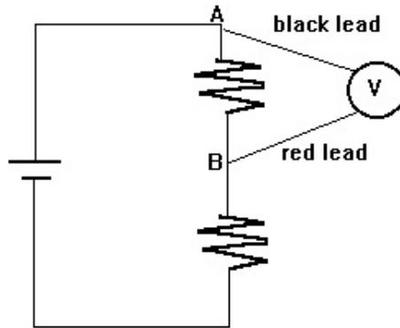
Notice how the voltmeter is connected "outside" the circuit. This meter is measuring the voltage from A to B and this is often called the voltage across the resistor. The voltage across the battery would require you to hook the meter up on each side of the battery.
