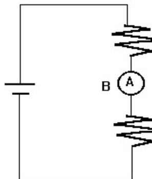
A few comments should be made regarding the positioning of the meter leads in the circuit. Consider the diagram below.
