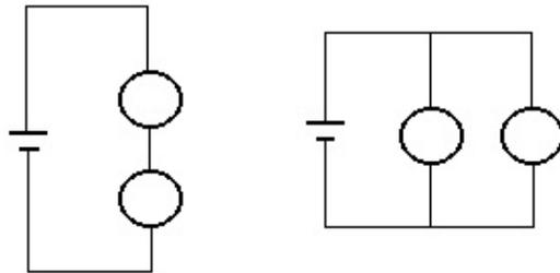
The set up on the left is called wiring the light bulbs in series and the set up on the right is called wiring them in parallel. Using your knowledge of circuits, you should be able to reach the following conclusions:
