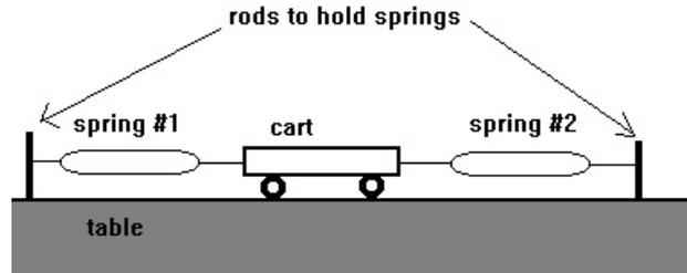
2.) Set the cart in motion and produce graphs of position, velocity and acceleration versus time.
