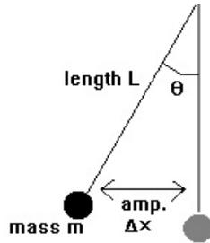
In this investigation we will only deal with small amplitudes (i.e. the angle theta should not be greater than  $40^\circ$ ).
