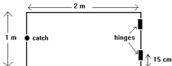
Suppose the door weighs 10 kg (the center of gravity is at the center) and it is set up so that when a 70 kg person (walking from right to left) lands at a point 0.5 m from the left edge, the catch will break (not before). What maximum force should the catch be able to sustain? What is the force on each hinge at the instant before the catch breaks? (T2\*)
