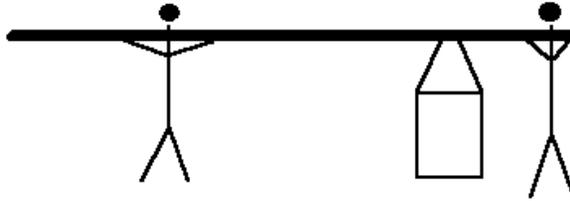
5.) A person wishes to carry a 3 m bar that weighs 100 N perfectly horizontal with a 500 N load on one end and a 300 N load on the other. Where should he or she hold it? (T8\*)
