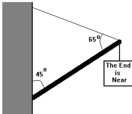
9.) A piece of modern art is to be hung in a gallery as shown below. The bar from which it hangs is 2 m long and weighs 100 N. The artist insists that it be hung from one string connecting the bar to the ceiling and that it must be balanced as shown or his commentary on the angst of modern life will be ruined (he says as he strokes his goatee). Exactly where on the bar must the shop keeper position the string? Note: diagram should say sign weight = 250 N.
