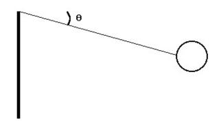
This dip causes two sources of error to occur in your lab. First the centripetal force is no longer equal to the weight of the washers, it is equal to Wcos $\theta$ . Second, the radius that was used to calculate your velocity and your slope is no longer a constant for each trial (r), but instead is equal to rcos $\theta$ , which is different for each trial (r is the string length).
