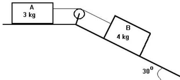
13.) Consider the set up as shown below. Using the quantities given (the coefficients of kinetic friction are next to each incline), determine:
