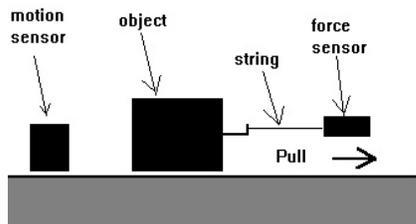
2.) After being sure the sensors are calibrated, begin the experiment by turning on the sensors and gradually increasing the pull on the force sensor until the object moves about one meter across the table.
