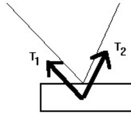
block supported by two strings attached at same spot.  $T_1, T_2$  not equal
