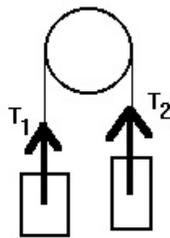
pulley system, same string.  $T_1 = T_2$
