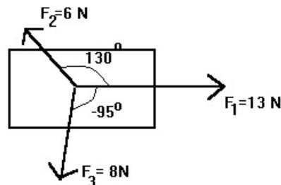
Notice how all the forces are drawn from the center of the object and all angles are measured relative to the horizontal (+x) axis.
