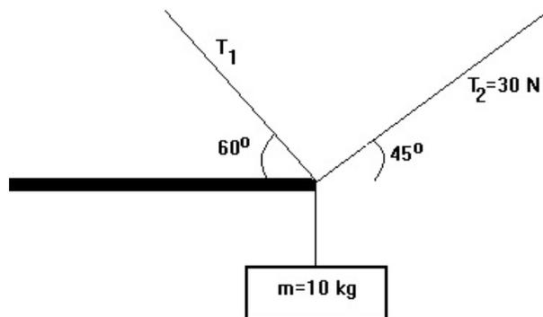
4.) Determine the mass of  $m$  that will keep the system below in equilibrium (all surfaces are frictionless). (010)
