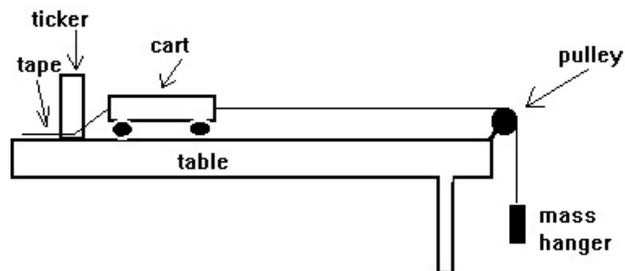
2.) Place 400 g of slotted masses on the cart. When the procedure calls for you to put a mass on the mass holder, use the masses on the cart. It is important that the masses on the cart and on the holder add up to 400 g at all times (there is a reason for this will be apparent in a few chapters).
