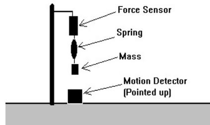
2.) Set the mass in motion and begin recording data from both the motion detector and the force detector. Continue for five or six full cycles of the masses motion. If the motion detector is not registering properly, put a piece of cardboard on top of the mass to give it a better reflecting surface.
