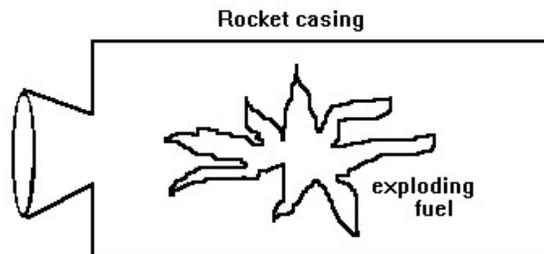
Thus we see that the principle behind a rocket engine is actually very simple (the implementation and efficiency is another story), and we see how rockets don't "push off" the launch pad, they don't really need a launch pad at all. The fuel pushes the engine up and the engine pushes the fuel down and out.
